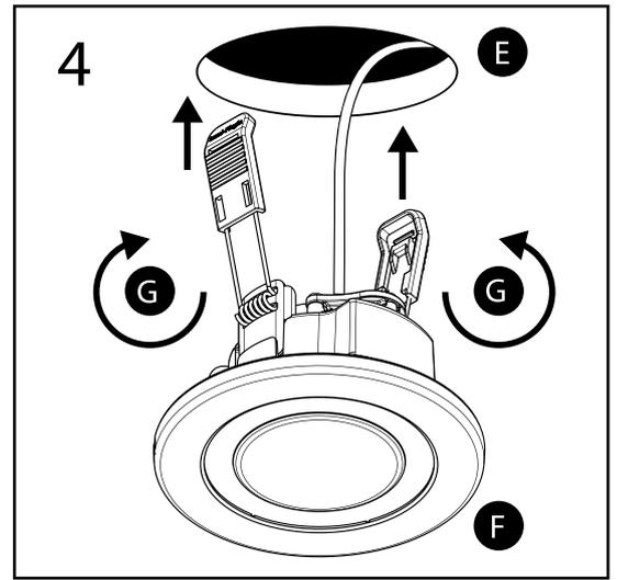
**A** Ceiling surface **B** Mains supply **C** Live / Neutral cable **D** LED Driver **E** LED Driver output cable **F** Lumi-Plugin Downlight **G** Spring clips
